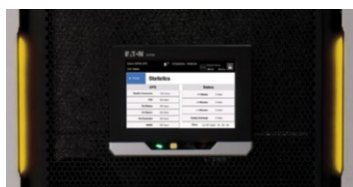
Yellow light bars indicate battery or bypass.
